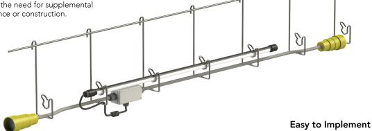
Each segment allows for rapid deployment of 150 feet of tunnel wall lighting with (10) 4' VPX fixtures spaced every 15'.
