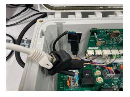
Switch the RELAY CTRL SOURCE switch on the Slave PDT board(s) from CW to INT
